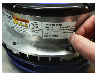
Sticking the EM-W inside label on the ECblue housing.
